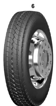
Design of four consistent grooves and slant-edge pattern provide outstanding drainage and grip performance Design of Broader tire shoulder improves tire's abrasion resistance and longer tire mileage Special tire shoulder design, low heating formula to decrease shoulder heating, increase tire durable performance. Low rolling resistance, Save fuel consumption, and excellent handling performance.
