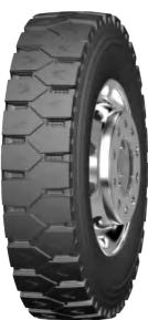
Interlaced reinforcing rib design at the pattern block bottom provides better tear resistance and anti-puncturing performance; Stone emitter at the bottom of grooves protects tire carcass effectively. Improved traction, driving and braking performance
