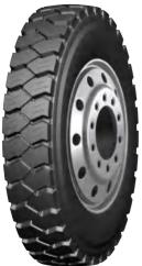
Interlaced reinforcing rib design at the pattern block bottom provides better tear resistance and anti-puncturing performance; Stone emitter at the bottom of grooves protects tire carcass effectively. Improved traction, driving and braking performance With strong ground grip, good self-cleaning, good standing wear and high in loading ability
