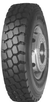
Design of wide rib grooves with lug grooves provides better water dispersion, improves driving and wetresisting performance Design of pattern blocks offers excellent traction performance. Open groove and bottom design given excellent self-cleaning performance Reinforced bead and body to strengthen the puncture resistance, tear resistance. Open shoulder and block type pattern provides strong traction and gripping stress.
