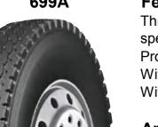
Three zigzag grooves design and Combination of rib and lug design on shoulder ensure excellent heat dissipation and high speed performance
