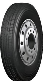
4 straight groove can provide superior braking and driving performances, superior adhesion properties of the ground, excellent wet skid resistance, eccentric wear resistance
